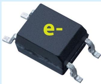
**“Nuclear” battery converts the energy of the beta decay of Carbon-14 into electric power by means of converters based on porous heterostructures “por-SiC/Si”**
