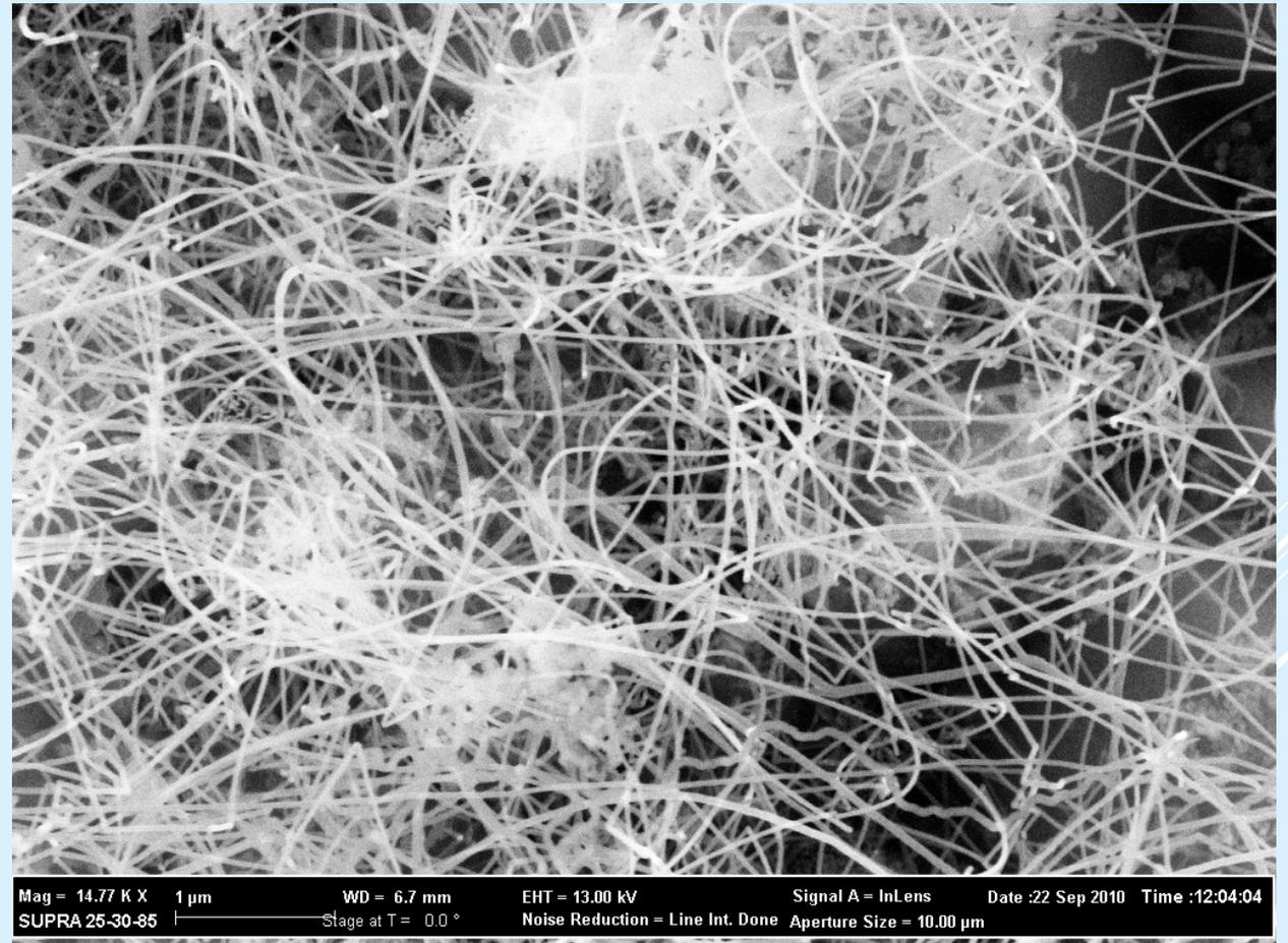
*Silicon carbide nanowires on the porous structure surface*
