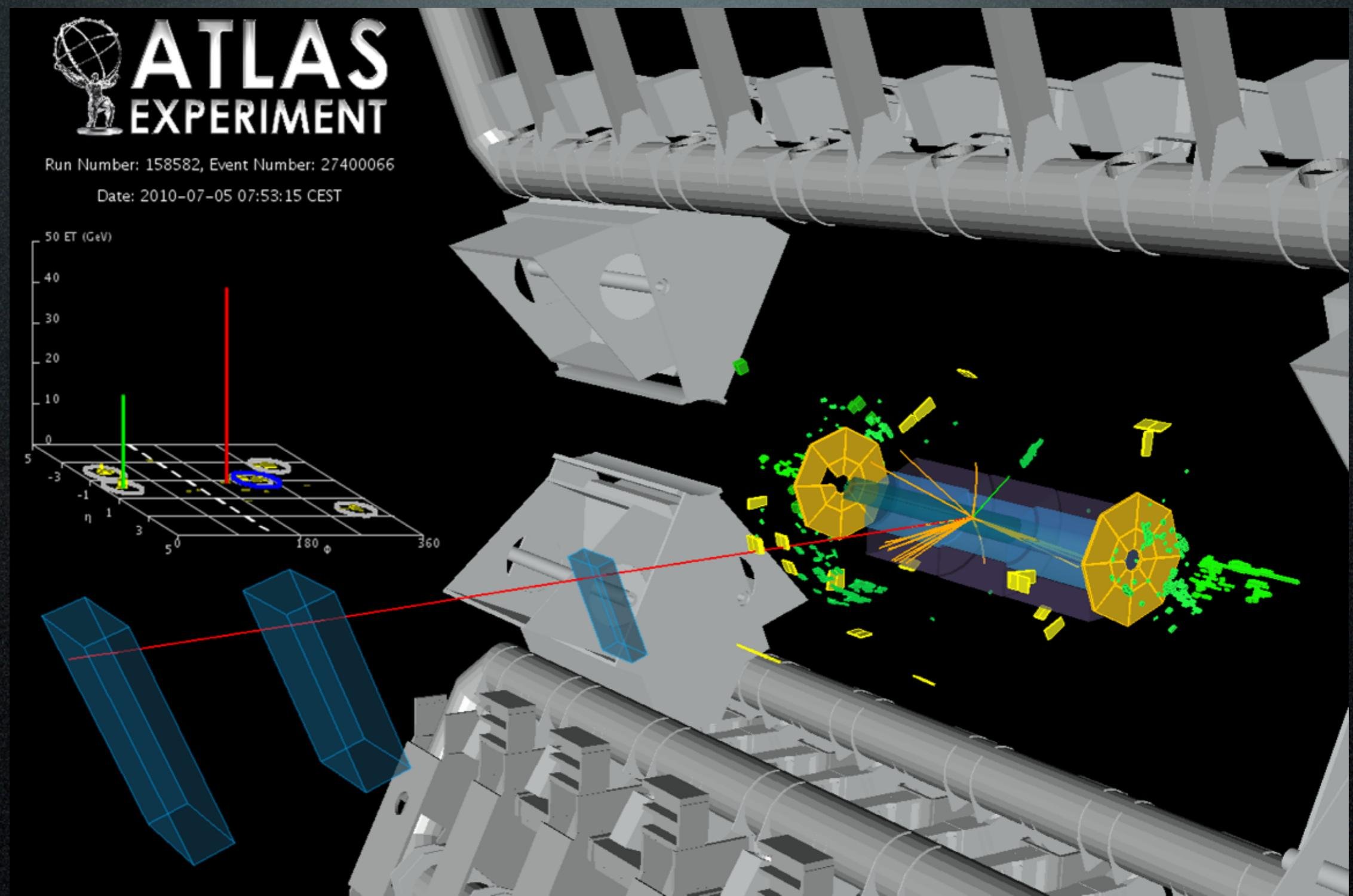
Red: Isolated muon track ( $p_T = 48 \text{ GeV}$ ) ; Green: isolated electron track pointing to a green Calo cluster ( $E_T = 23 \text{ GeV}$ )
