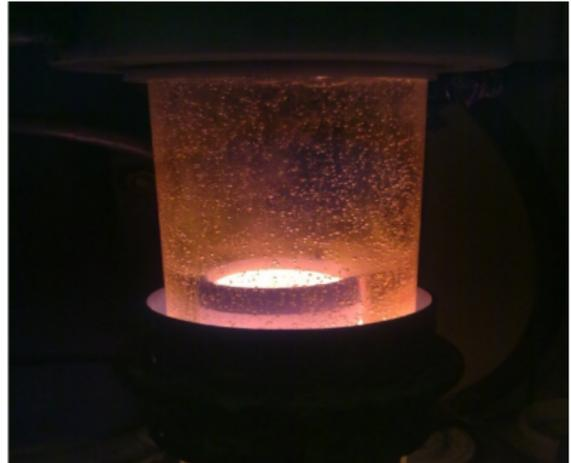
Pic.5. Schematic representation of chemical transport (experimental silicon substrates are indicated in orange); to the right: CVD endotaxy reactor of the SiC / Si family of heterostructures.
