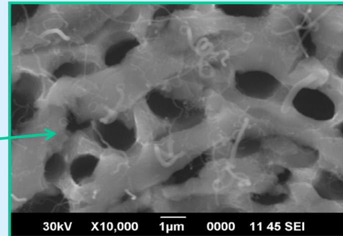
The wall thickness between the pores is 10-50 nm
