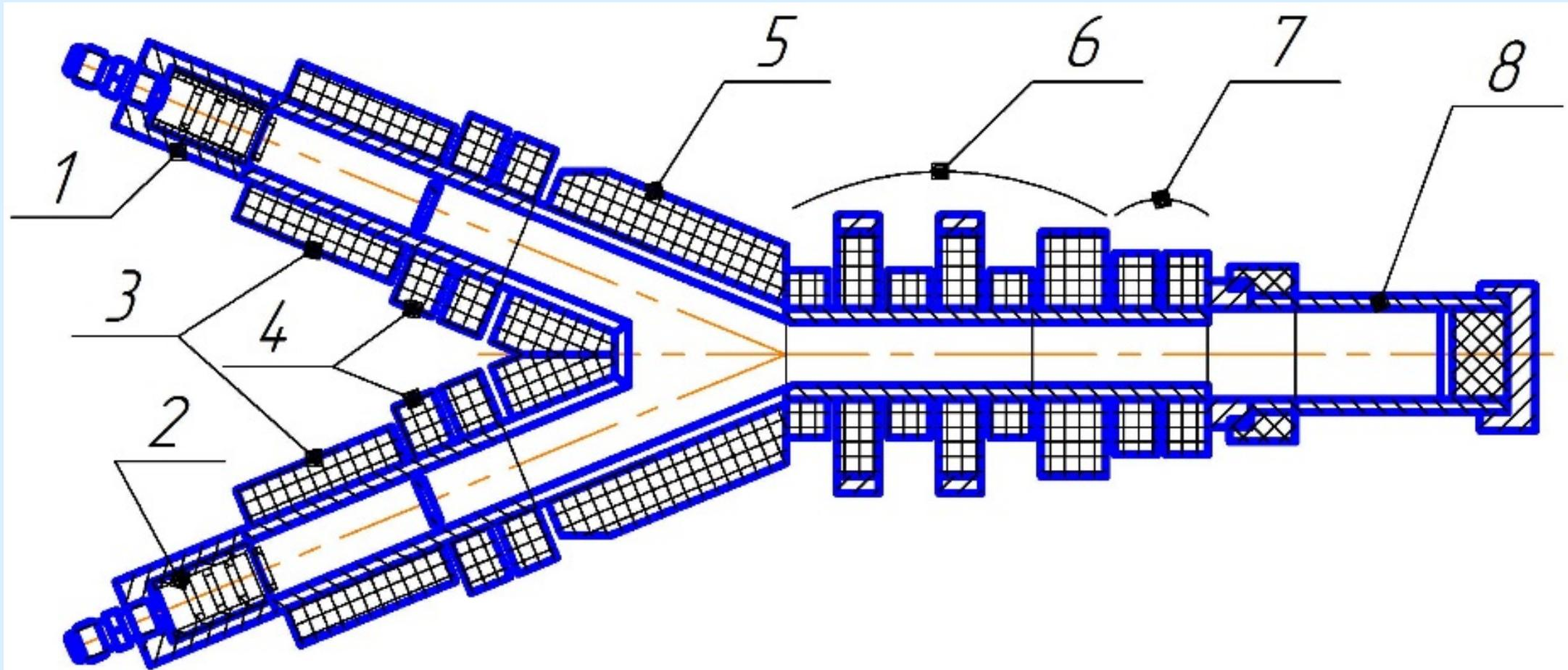
1- ionization lithium hydride LiH 2- ionization nitrogen 3 – injector 4 - Magneto-optical drive - driver 5 - Accelerator-driver
