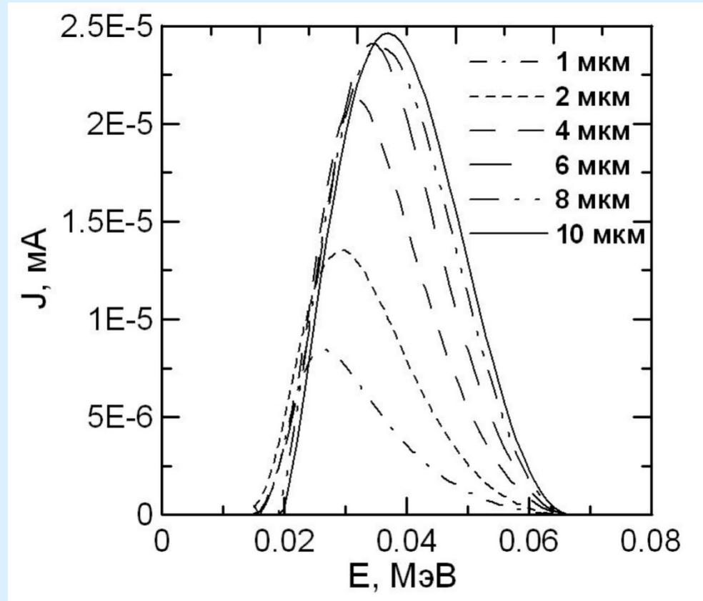
Current generating from the SCR spectrum width to depth  $p$ - $n$ -transition using isotope Ni-63 with an activity of 20 mCi.
