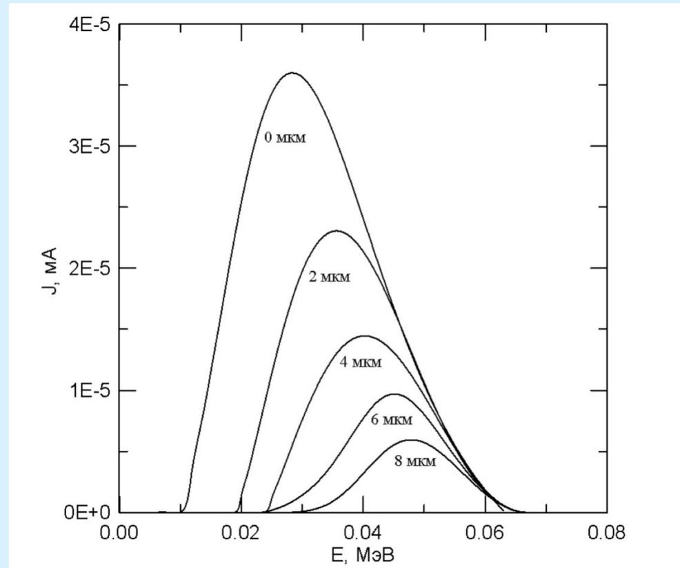
Spectrum generation current of depth  $p$ - $n$ -transition to SCR width 8 microns using the isotope Ni-63 with activity 20 mCi.
