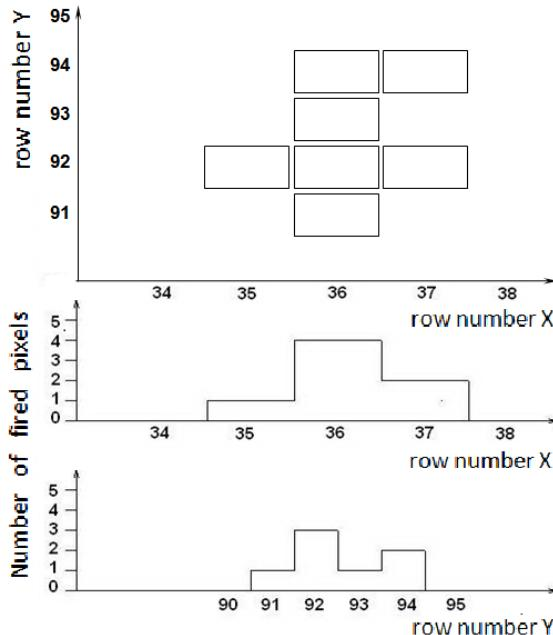
This picture presents a typical cluster structure in XY plane and its projections on both axes for the 3-rd of 8 cycles. To calculate particle position we use center of mass approach. In each projection the number of the row ( $n_X^i$ ), is multiplied by the number of fired pixels in this row ( $R_x^i$ ), and the sum of the products is divided by the total number of fired pixels in the cluster  $N_P$ :
