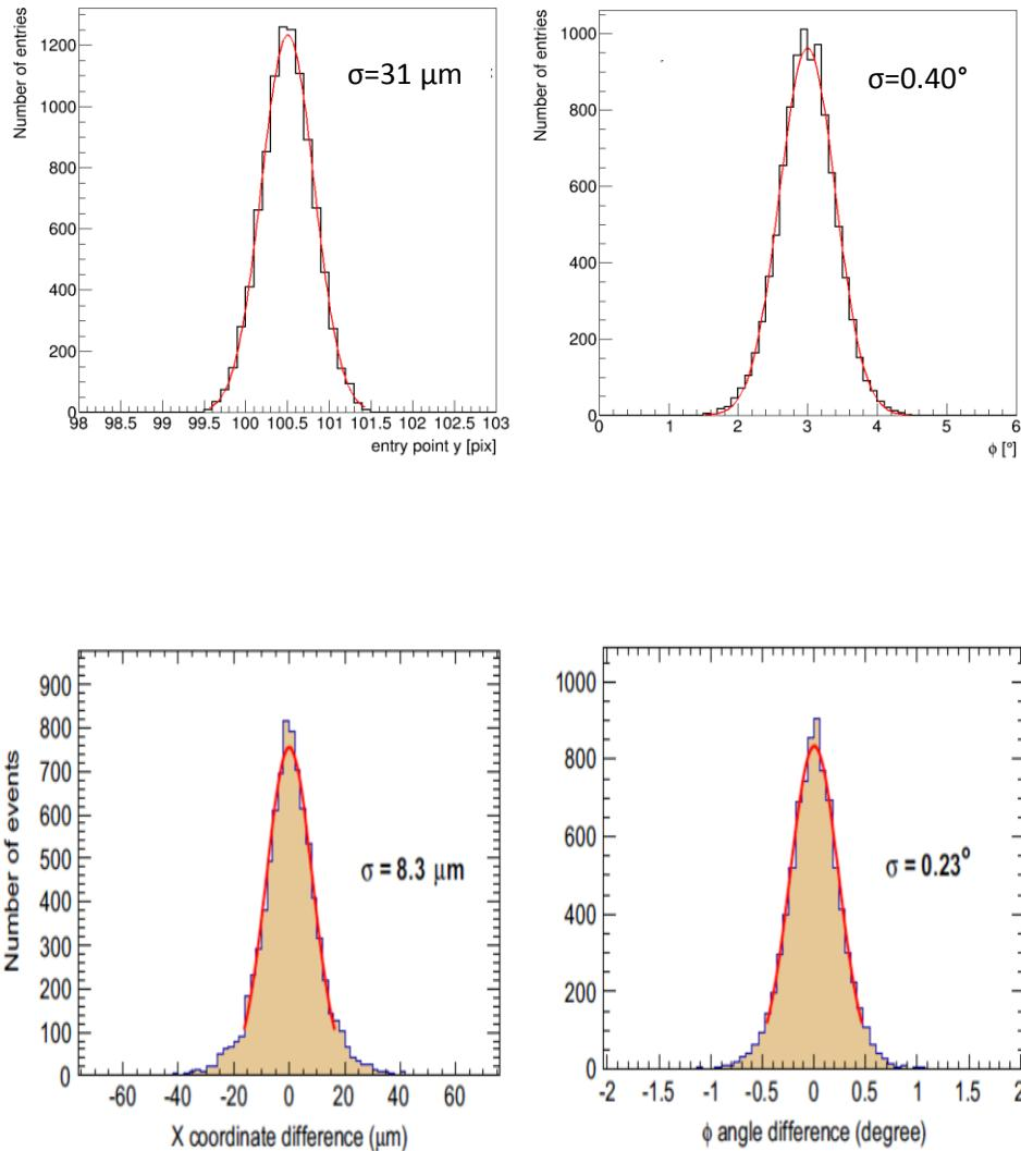
To estimate expected resolution MC simulations for different detector geometries and gas mixtures have been done.
