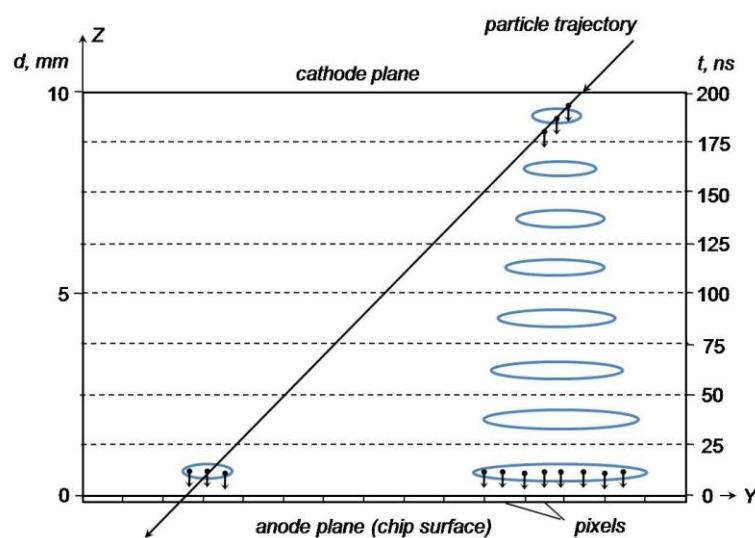
Electrons generated by an ionizing particle in a gas drift transversely towards the chip surface, where they are registered by the pixels of the chip every readout cycle.
