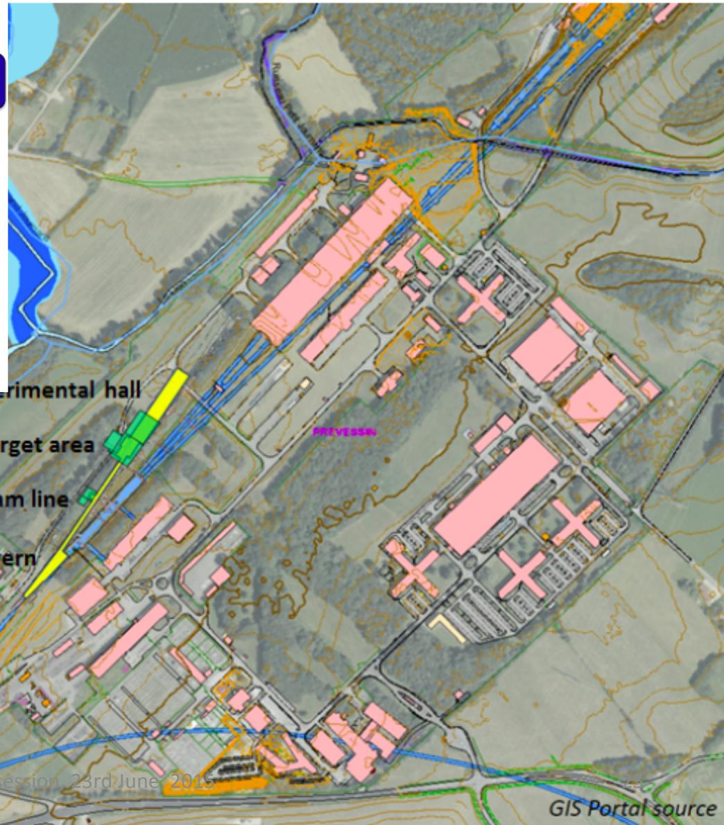
The SHiP facility is located on the North Area and shares the TT20 transfer line, and slow extraction, with the fixed target programmes
