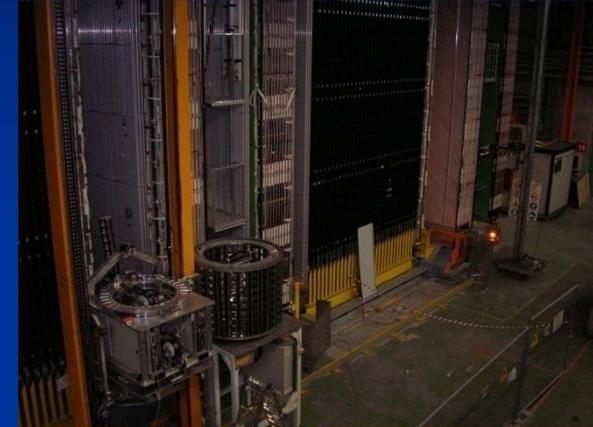
The Brick Manipulator System extracts the candidate brick from the wall
