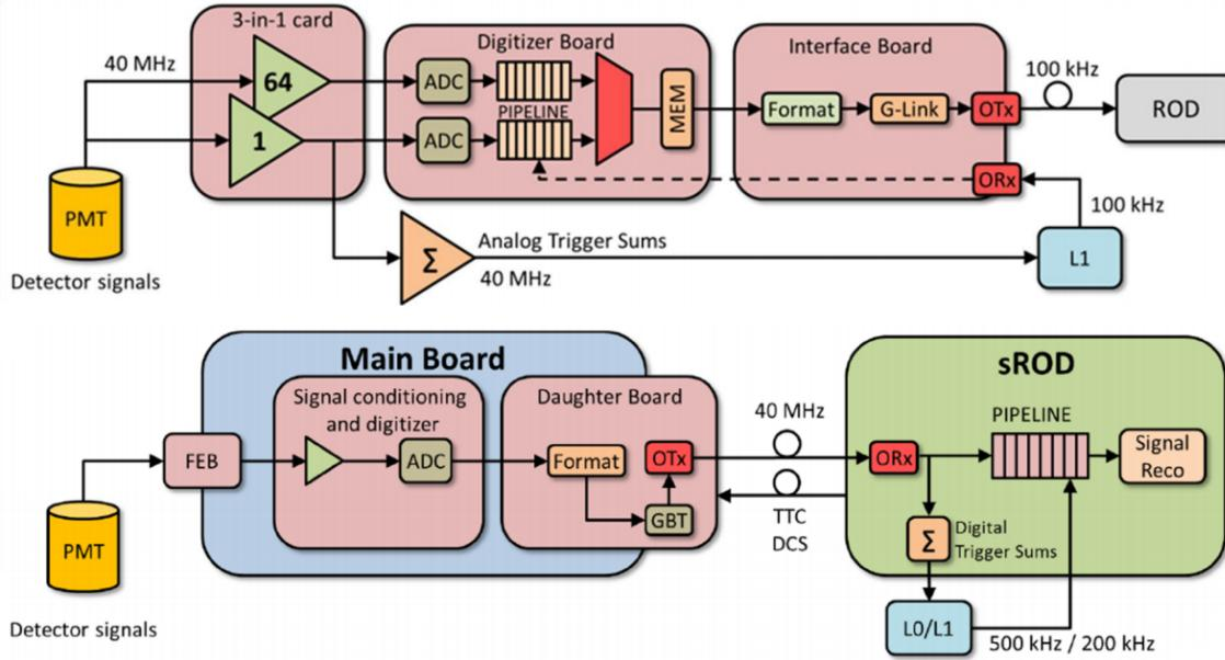
Figure 2: Current read-out structure (top) and new read-out structure (bottom).
