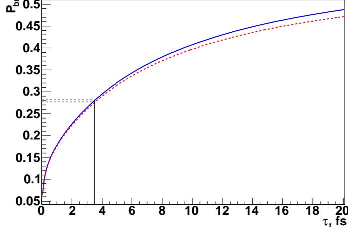
Figure 1: Dependence of the breakup probability  $P_{br}$  on  $A_{\pi K}$  lifetime for  $108\mu\text{m}$  (solid blue line) and  $98\mu\text{m}$  (dashed red line) nickel targets, and an example how lifetime could be obtained from experimentally measured breakup probability.
