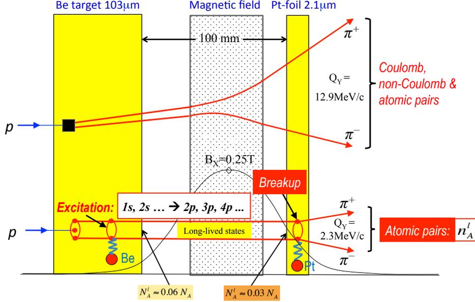
Figure 2: Method to observe long-lived  $A_{2\pi}^L$  by means of a breakup foil (Pt).
